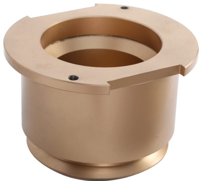
This is a rotating bushing assembly that has 3 bearing races that allow for the inner sleeve to rotate within the outer body. North Star uses 4140 HT & Quenched alloy raw material in the manufacturing of our rotary deck bushing, which provides high performance combined with longer service life.
